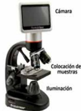
FIGURA 4: MICROSCOPIO DIGITAL PARA CAPTURAR IMÁGENES.
